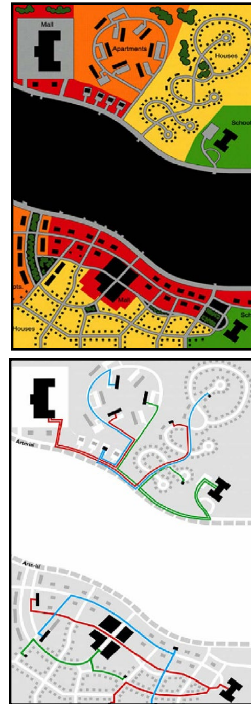
The lower part of each diagram shows how routes between destination points in a mixed-use area with gridded street network are more direct and result in fewer trips on the arterial network.
